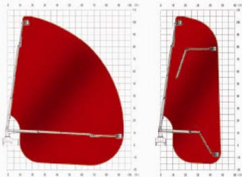
Even when short-jacked, the T-Rex allows vertical and horizontal reach above or below grade.
